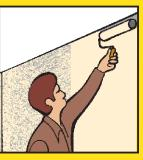
8. Apply 1st coat of saturant to adjacent area.
